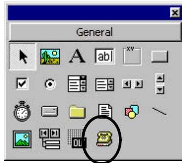
Figure 26.2 Toolbox showing Comms components.
